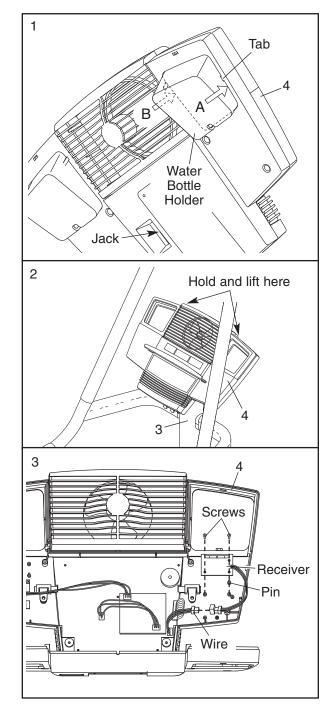
4. Refer to step 2 above. Lower the top of the Console (4) and the fan. **Make sure that no wires are pinched.**Reattach the top of the Console with the four screws removed in step 2. Refer to step 1 above. Press the water bottle holders back into the Console. If you removed a silver ring from the audio cable jack, reattach the silver ring.
